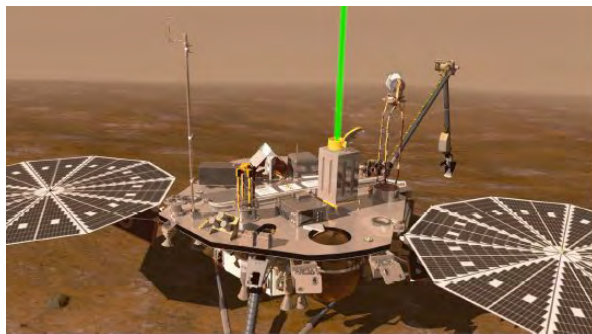
Figure 3. Artists impression of the Phoenix lander clearly showing the lidar and MET mast.
